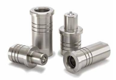
DSE Series poppet style couplings are the most common design used in subsea applications and can be connected and disconnected at full system pressure. Typically connected and disconnected above water, their compact design is efficient and reliable.
