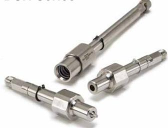
DSH Series couplings are used in subsea and topside RBJ-Plates. Typically found in hydraulic pilot applications they replace legacy couplings, pipe nipples, and fittings eliminating potential leak paths and reducing assembly time. The superior valve design of he DSH Series accomodates plate flex up to 0.100 in/2.54mm.
