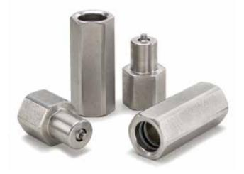
DSA and DSU Series poppet couplings are used in many subsea and topside applications. The ability to connect and disconnect under full system pressure, and sealing that can withstand internal and external pressure, provides secure connections for a variety of applications.
