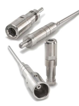
DSC Series are traditional subsea couplings with PEEK seals. Redundant sealing adds a higher level of integrity to this proven design. The guide sleeve eases alignment of the coupler and nipple for a smooth connection.
