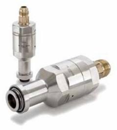
DSS Series swivels provide an unobstructed flow path force balanced design and low friction PTFE slipper seals minimize rotation torque. These features minimize pressure loss, can increase hose life and reduce fitting loosening.
