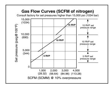
All RVP models are designed primarily for thermal expansion or low volume relief applications at high pressures where flow is not critical. Thus, liquid curves for these models are not shown.
